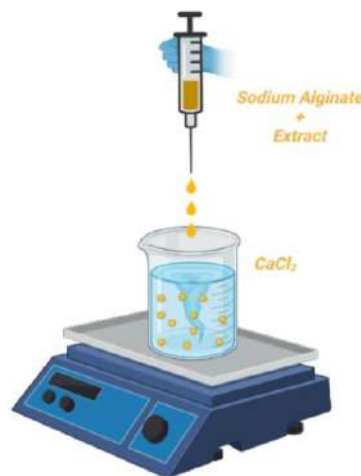
Figure 1. The schematic representation of alginate beads preparation by ionic gelation method
